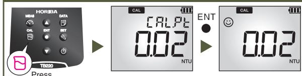
4. Repeat steps 2 and 3 for each standard solution vial. After completing the four calibration points, the screen will switch to measurement mode.
