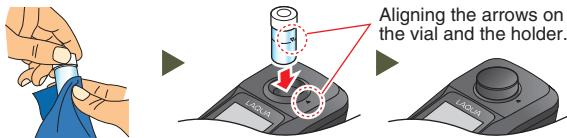
3. Press the MEAS key to start measurement. When the symbol stops blinking, record the reading or press the ENT key to save the data.
