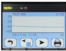
The value of the current measurement at the red cursor line is shown on the right side of the top bar area.
