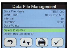
The *Data File Management* function allows the user to inspect how the data was captured and other file attributes. It also allows the possibility to delete the file and also ALL files associated with the *Location ID* but not the *Location ID* itself which will be saved ready for another logging event.
