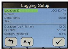
There is provision for 20 *Location IDs* to be held on the SDHmini-L. Here is an example of how to create a new Location ID called TEST.
