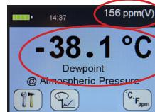
Here the secondary display is being changed to ppm(v) engineering units (B).
