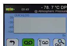
To run data logging events with different durations and sample rates to the default setting and with the ability to attach alternative names or Location IDs, press the *Configure Data Logging* key to enter the *Logging Setup* screen. The *Location ID* or file name may be specified here as well as the sample interval and the number of data points.
