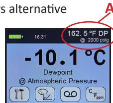
To choose the engineering units to be displayed, select the units key  ${}^{\circ}\text{F}_{\text{ppm}}$  from the main digital view.
