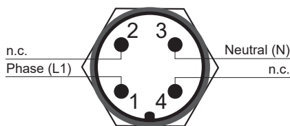
Fig. 36 Plug for power supply 100 - 240 V AC on polycarbonate enclosure, front view
