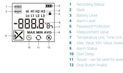
By pushing the green start button 🜔 in quick succession, further information can be accessed on different pages of the display. The display changes from the current temperature display first to the maximum recorded temperature value, then to the minimum and lastly to the average value of the current recording.
