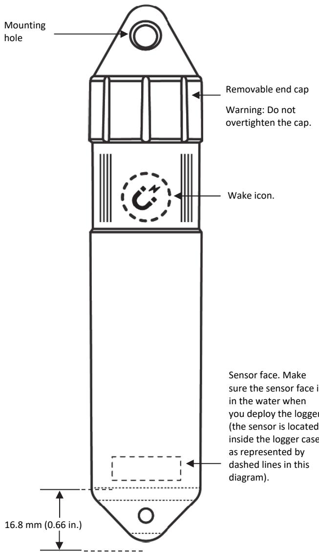
**Important:** When storing or transporting the logger, keep the magnetic fob (or any other magnet) a minimum of 1" away from the logger so that you do not inadvertently drain the logger's battery.
