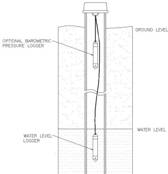
5. Measure the water level from the desired reference point (e.g., top of pipe, ground level, or sea level).
