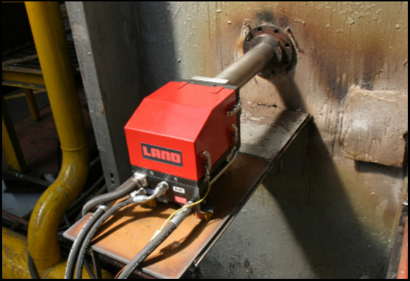
Typical installation showing the FTI-Eb mounted into a process - the sensor is shown in the protective enclosure
