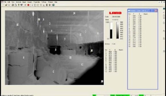
Point temperature measurement inside the furnace
