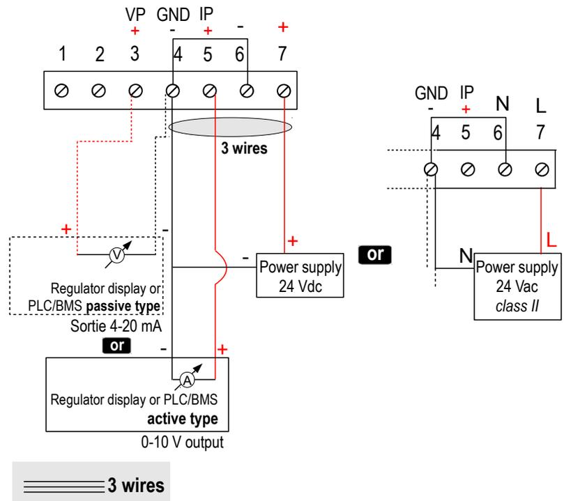
For CP112/113 – PO models and CP112/113 – PN models with 4-20 mA output – **passive** :
