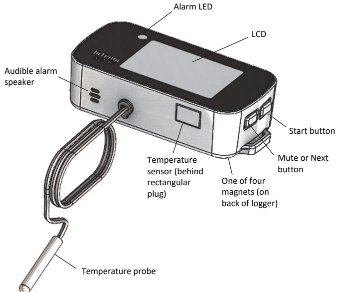
**Start Button:** Press this button for 1 second to start the logger when it is configured to start “on button push.”
