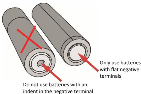
To install or replace the batteries:
