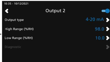
Activate the output tapping
