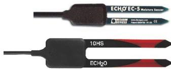
Soil moisture smart sensors are used for measuring soil water content and are designed to work with smart sensor-compatible HOBO® stations. They combine the innovative ECH<sub>2</sub>O® Dielectric Aquameter probe from METER Group with Onset's smart sensor technology. All sensor conversion parameters are stored inside the smart sensor adapter so data is provided directly in soil moisture units without any programming or extensive user setup.
