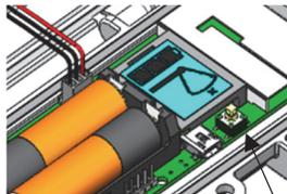
Open the sensor node door and install the rechargeable batteries. Press this button on the sensor node for 3 seconds.
