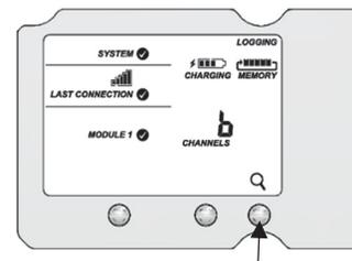
Press the Search button on the station again to stop the search for sensor nodes.
