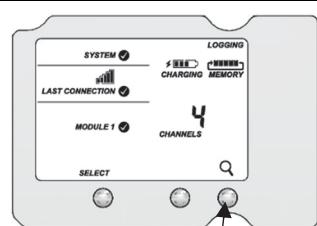
Press the Search button. The magnifying glass icon blinks while the station is in search mode waiting for sensor nodes to join the network.
