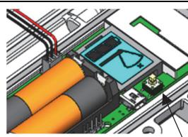
Open the door and install the rechargeable batteries. Press this button on the sensor node for 3 seconds.
