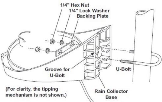
4. Slide the metal backing plate over the bolt ends as they stick out toward the rain collector cone. Secure the backing plate with a washer, a lock washer, and a hex nut on each of the bolt ends. Adjust the height of the rain collector, then tighten the nuts.
