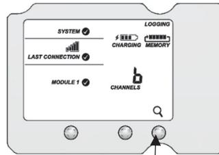
Press the Search button on the station again to stop the search for sensor nodes.
