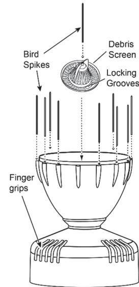
2. Place the cone back onto the base by putting the latches on the cone into the latch openings in the base and rotating the cone clockwise until the latches "lock" into place.
