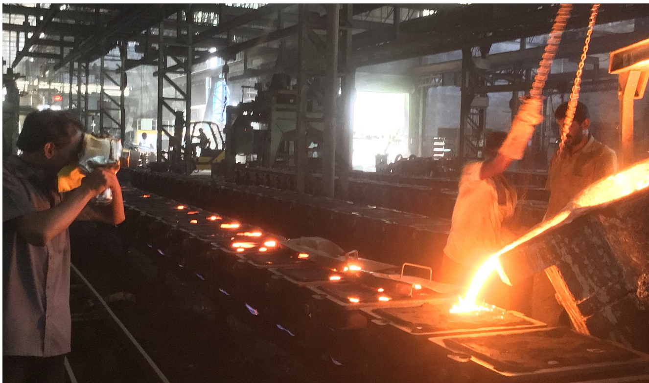
Measurement taken while pouring liquid metal into the moulds - Manual Pouring Lines.
