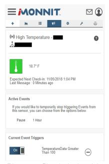
You can toggle the Event Trigger on or off by selecting the switch under Current Event Triggers.
