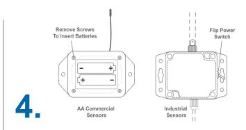
Insert batteries or use the switch to power on the wireless sensors.
