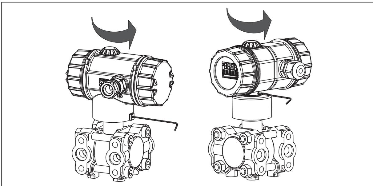
1. Loosen the threaded pin using a 1.5 mm hex wrench.
