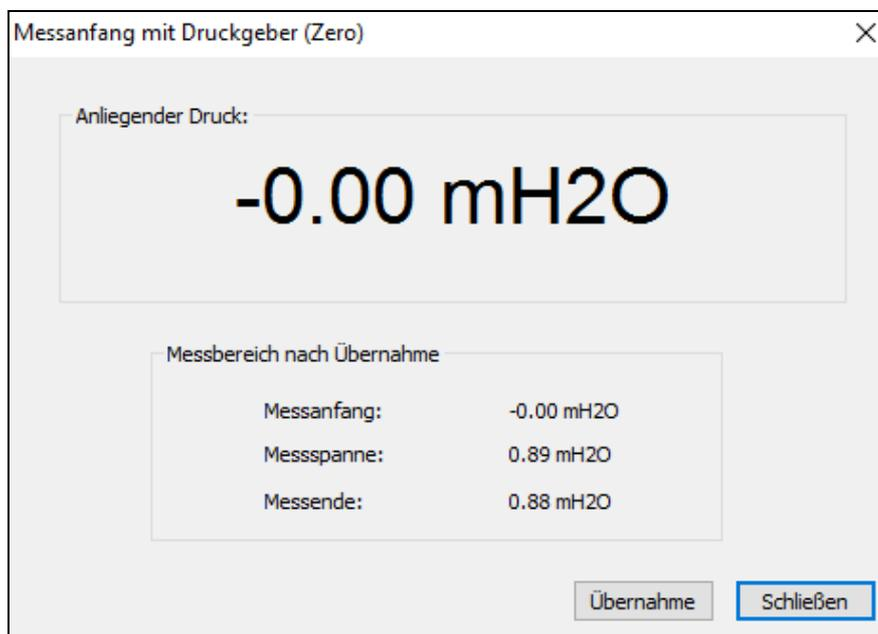
**Extras**      **Extras: Online operation\_measuring end with pressure transmitter (span)** – with full tank
