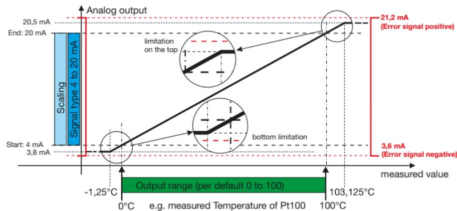
In this example, the measured value from 0 to 100°C is output on the analog output with 4 to 20 mA.
