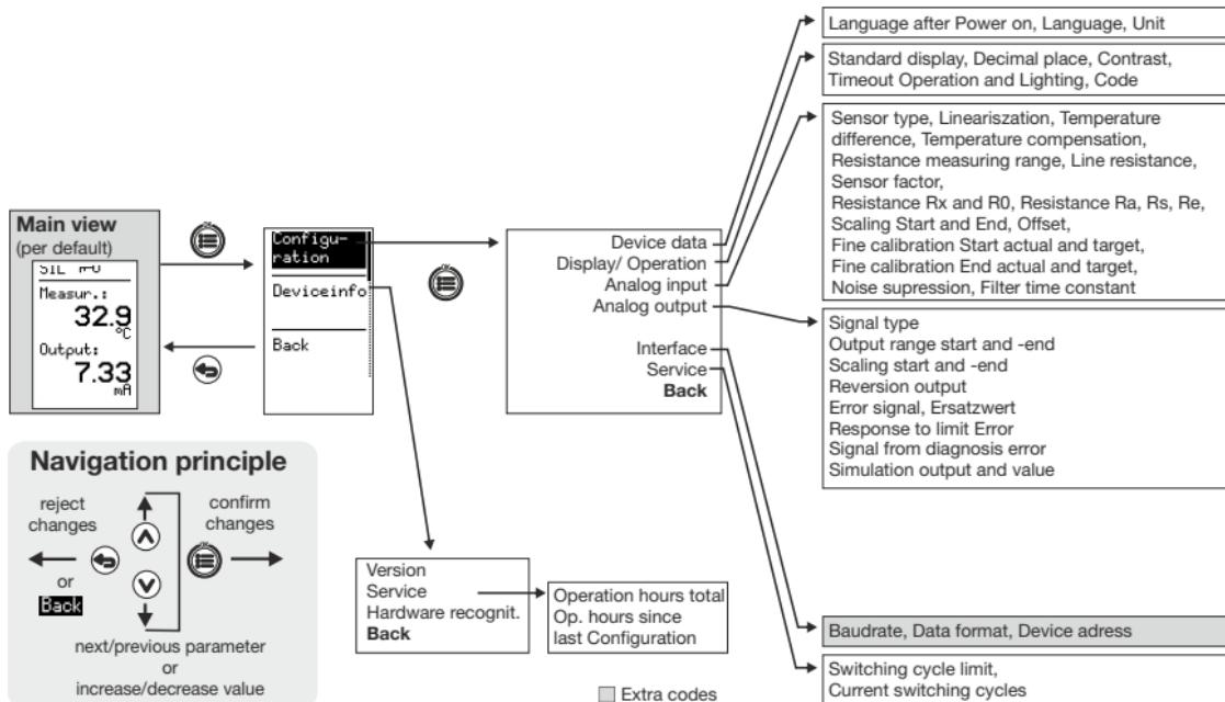
All the parameters are freely accessible, but they can be locked via a code on the device or with the setup program. Default settings are shown in **(bold)**. All parameters are listed in the following tables. Parameters which are not required are automatically hidden depending on the setting.
