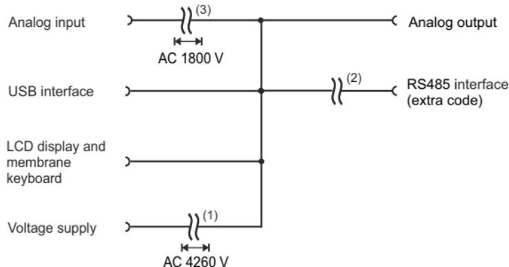
(1) The voltage specifications correspond to the alternating test voltages (effective values) according to EN 61010-1:2011-07 for type testing.
