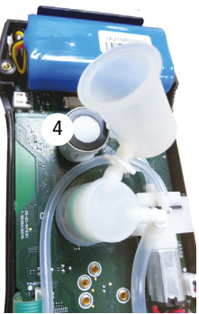
New sensor connected to electronic board
