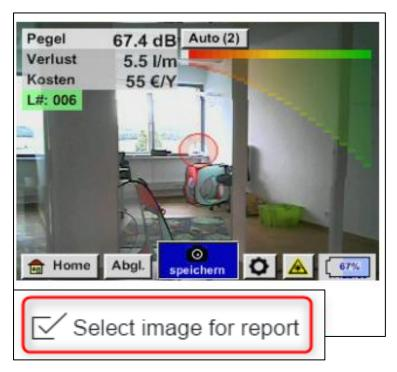
If there is any additional image from another device/camera available, this can be added to the existing picture. Using the checkbox below, the original leak detector image could be replaced with the selected picture and marked for printing it in the report for the specific leak.
