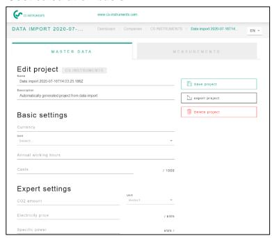
If the electricity price and specific power were filled in the expert menu, the electrical costs of the compressed air system get calculated automatically.
