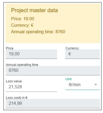
This figure shows the data with which the system calculates the costs. The yellow block displays the parameters of the project master data, and they cannot be changed during local measurement.
