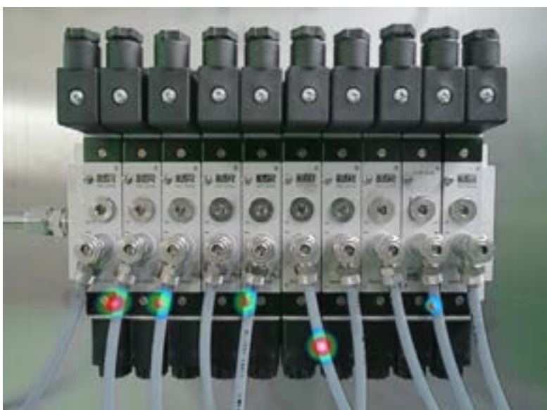
LeakCam 600 with 64 microphones (Power Beam Forming)
