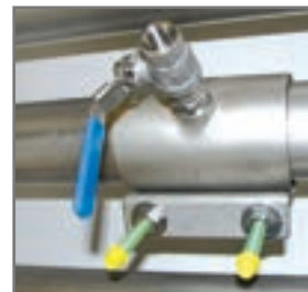
B Spot drilling collars
