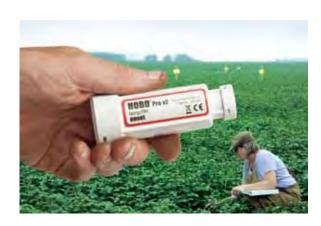
HOBO Pro v2 data loggers are weatherproof loggers that provide high accuracy temperature and relative humidity measurements in a wide range of outdoor environments.
