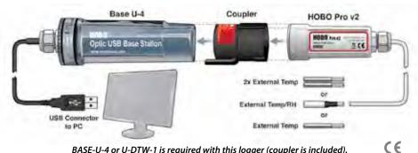
BASE-U-4 or U-DTW-1 is required with this logger (coupler is included).
