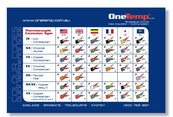
**Thermocouple Wire:** Twin, single conductor, having a temperature/E.M.F. relationship to the appropriate standard over the complete temperature range.
