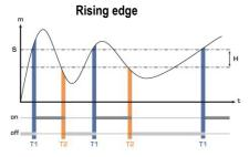
Measurement (m) > Threshold (S) during the time-delay T1 → Alarm activation
