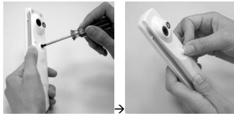
⚠ Since the thermometer is splash proof, please make sure the battery cover is tight for the thermometer and also with the rubber gasket.
