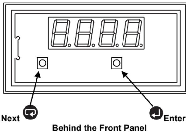
The instrument uses a single level menu structure. The menu system lists *parameters* (eg. **inPt**, **unit**, **dP**, etc.), each of which leads to a list of configurable instrument *options* (eg. the parameter **inPt** leads to the options **mV**, **mA**, **Volts** etc.).
