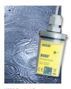
HOBO Pendant Event 7.1 x 3.3 x 2.3 cm (2.8 x 1.3 x 0.9 in) Cable 1.8 m (6 ft) 50 g (1.7 oz) The HOBO Pendant Event data logger is ideal for rainfall logging and connects to most standard tipping-bucket rain gauges to determine rainfall rates, times, and duration.
