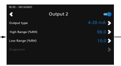
Activate the output taping —. Set the output type and high and low range values then tap the back arrow on the top left.
