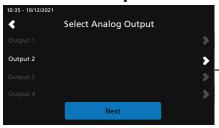
Tap the output to set corresponding to the previously configured channel.
