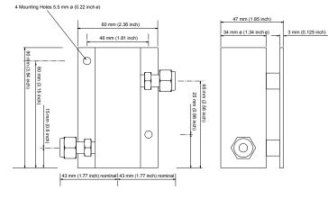
NOTE: The assembly is shown with 1⁄2 inch OD tube fittings. The dimension across the tube fittings will vary for all other size fittings.
