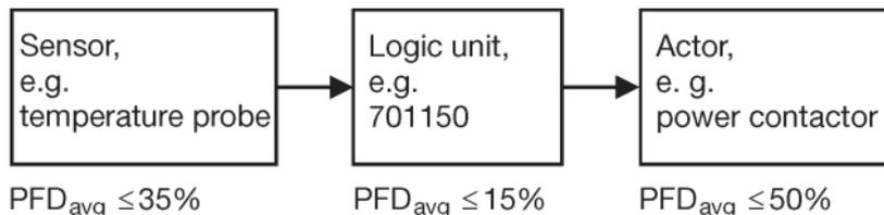
Typical subdivision of the "average probability of dangerous failures of a safety function on demand" ( $PFD_{avg}$ ) into subsystems
