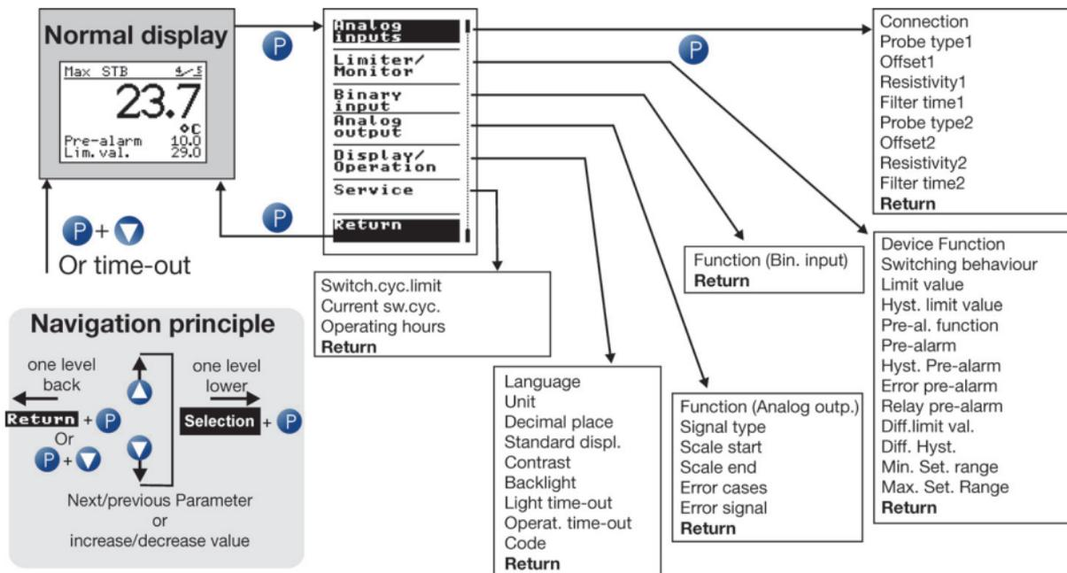
All the parameters are freely accessible at the factory, but they can be disabled via the setup program.
