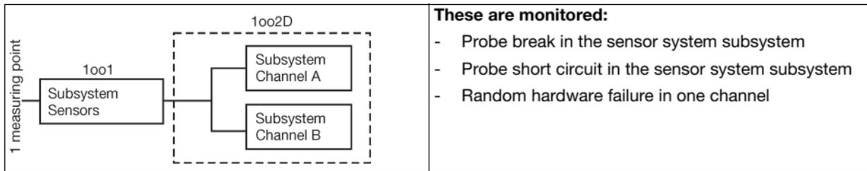
The variants with two sensors are consistently structured with two channels.
