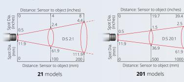
All models can measure at longer distances than shown, with a larger measured spot size.
