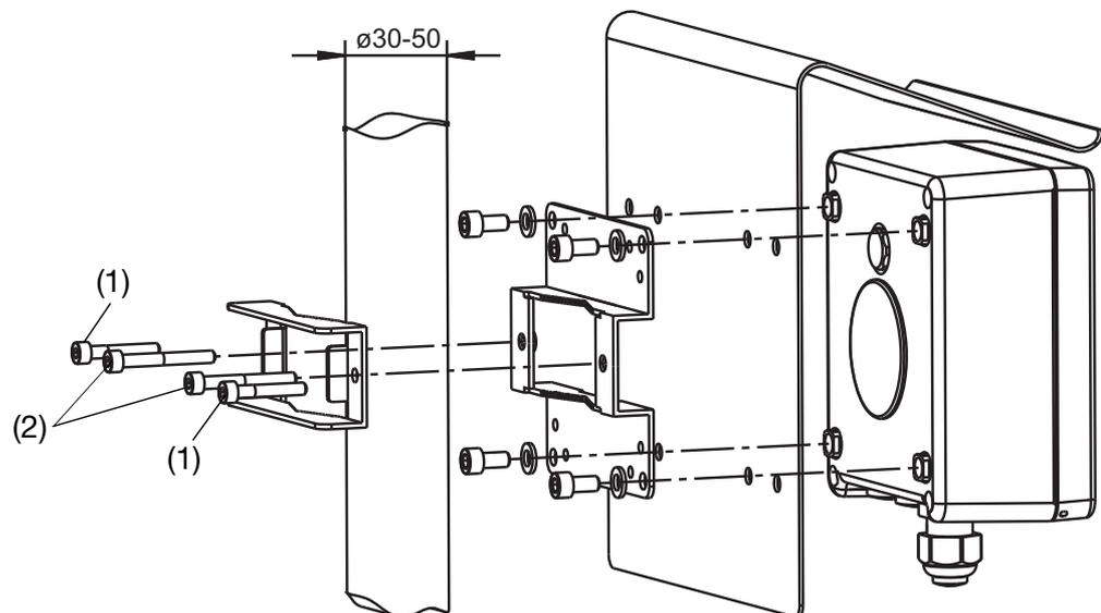
The M5 × 30 screws (1) are for pipe diameters of 30 to 40 mm.
