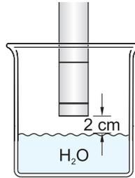
Make sure there are no drops of water on membrane. The sensor must remain dry during measurement. The use of a holding device (e.g. a test tube) is recommended.
