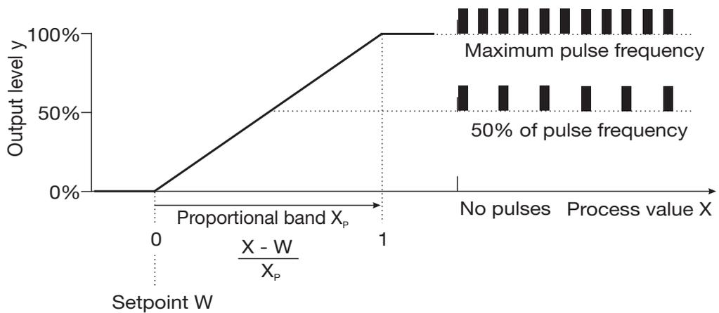
If the actual value  $x$  exceeds the setpoint value  $w$ , the P-controller controls in proportion to the control deviation. When the proportional band is exceeded, the controller operates with an output level of 100 % (maximum switching frequency).
