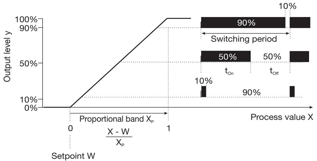
If the actual value  $x$  exceeds the setpoint value  $w$ , the P-controller controls in proportion to the control deviation. When the proportional band is exceeded, the controller operates with an output level of 100 % (100 % cycle ratio).
