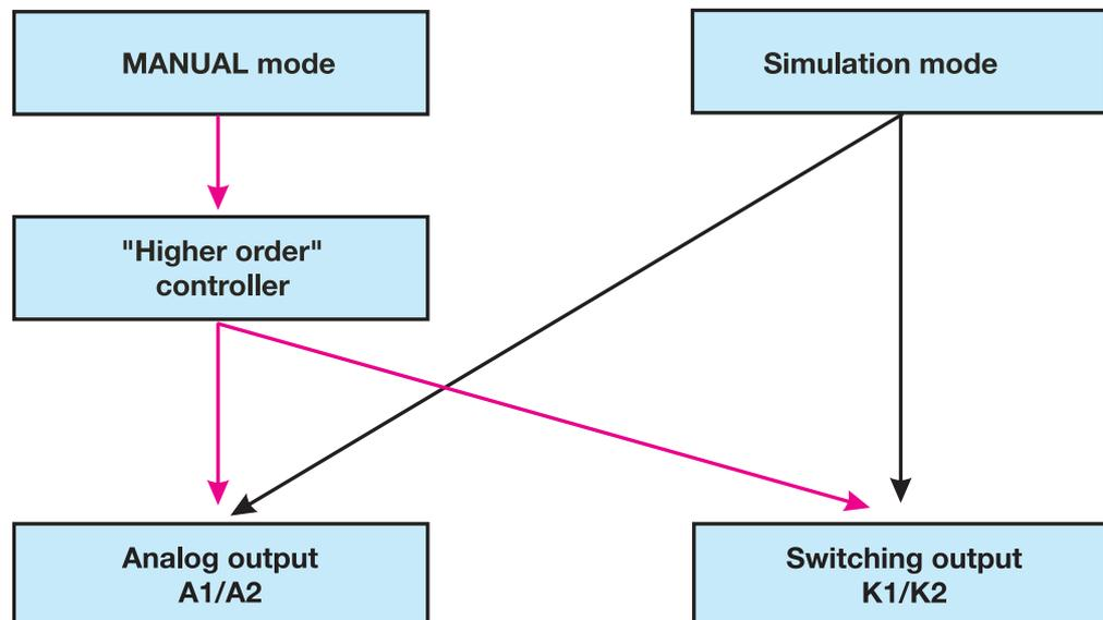
Simulation mode accesses switching outputs K1/K2 and analog outputs A1/A2 **directly**. If simulation mode has been selected, MANUAL mode **cannot** be used.
