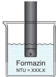
The device suggests the reference value "100.0 NTU" (flashing) for the calibration of the measuring range (0 to 200 NTU) selected in this example.
