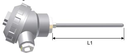
Large Alloy Head, Ceramic 3 way block, PT100 Class A, 6.4mm OD 316 Stainless Steel stem. Max Temp 260°C.
