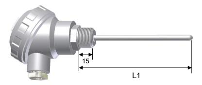
Large Alloy Head, Ceramic 3 way block, PT100 Class A, 6.4mm OD 316 Stainless Steel stem. Max Temp 260°C. ½" BSPT Standard.
