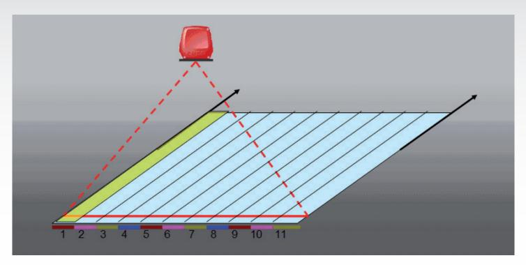
The chosen lane positions and sizes can be displayed above the product's thermal profile This way it's easy to check that the lanes are positioned correctly.
