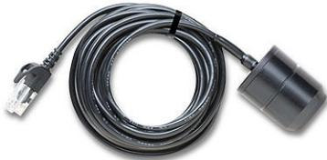
The silicon pyranometer smart sensor is designed to work with HOBO® stations. The smart sensor has a plug-in modular connector that allows it to be added easily to a station. All calibration parameters are stored inside the smart sensor, which automatically communicates configuration information to the logger without any programming, calibration, or extensive user setup.
