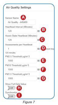
Note: Be sure to select the Save button anytime you make a change to any of the sensor parameters. All changes made to the sensor settings will be downloaded to the sensor on the next sensor heartbeat (check-in). Once a change has been made and saved, you will not be able to edit that sensor's configuration again until it has downloaded the new setting.
