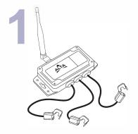
Remove your sensor from the package and install the antenna.
