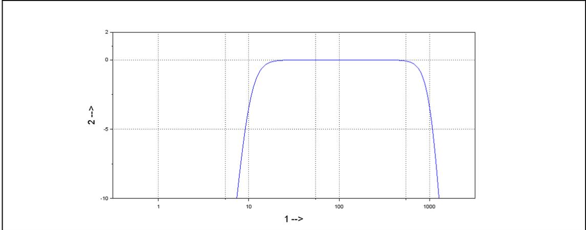
*Fig. 1: Typical frequency response 10 Hz–1000 Hz*
