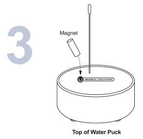
Use the included magnet to turn on the Water Puck as shown in the illustration. See a diagram of the light sequence on the next page.
