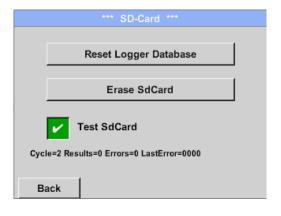
With activation of *Test SdCard* data are written and read to and from the SD-card.
