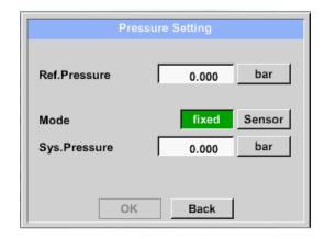
By using an ext. pressure sensor, which is detected automatically e.g. here at input B1, the button *Sensor* has to be activated.
