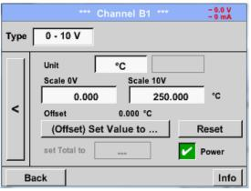
It is possible to define an Offset-Value. With the *Set Value to-*button (*Offset*) you enter it. The positive or negative difference of the *Offset* will be displayed.
