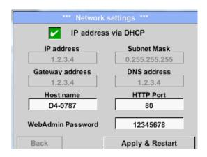
In the text description field *WebAdmin Password* could the password be set up. The password length is >=8 characters.
