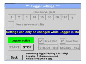
After the start and stop time activation and the created settings, the *Start* button will be pushed and the data logger is armed.
