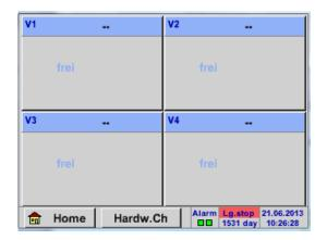
After pushing the button "Virtual Channels" in the Sensor Settings menu an overview with the 4 available "Virtual Channels" is displayed.
