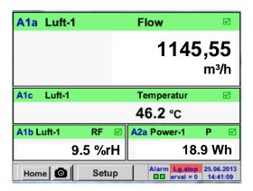
The view *Real time values* allows to display of 1 to 5 free definable measurement values.
