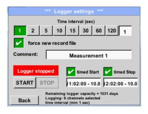
By pushing the *timed Stop* button and then the date/time description field below, the date and the stop time can be set for a data logger recording.
