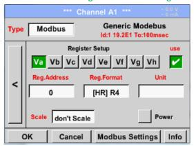
The measurement values are kept in the registers of the sensor and can be addressed via Modbus and read by the DS400.
