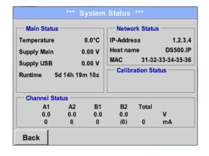
The function System Status offers an overview, fitting voltages and currents on the individual and the entire channels, as well as the power supply of the power supply units.
