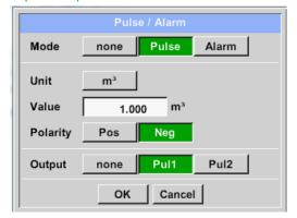
Select the impulse output using the "Imp1" or "Imp2" key.
