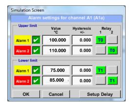
E.g., set the *Alarm 1* to relay 1 and the *Alarm 2* to relay 2.
