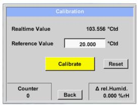
Here, a one-point calibration can be performed.
