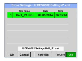
With Export system settings, all existing sensor settings can be exported to a USB stick or to the internal SD card. It stores all sensor settings including recording-, alarm-, graphics-, value-and name definitions.
