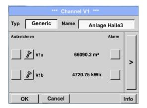
Result in *V1b* is the energy consumption read out from the energy counter.
