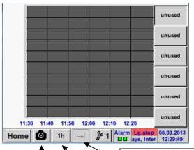
One or more channels for the recording and presentation of measured data can be selected here, such as a dew point sensor or several different sensors.
