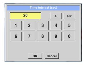
A different, individual *Time interval* can be entered in the highlighted white description field right at the head, where the currently set *Time interval* is always displayed.
