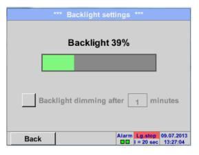
Here you adjust the desired *Backlight* (15-100%) of the display directly.
