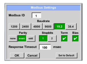
Please insert here the specified *Modbus ID* of the sensor, allowed values are 1 - 247, (e.g., here *Modbus ID* = 22)
