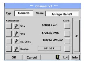
Calculation of the *specific. Perfor.* Is done in V1c with V1c = V1b / V1aFor this example, it is 0,072 KWh/m<sup>3</sup>
