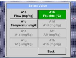
Pressing the respective channel button e.g. *A1b* will select the measurement channel
