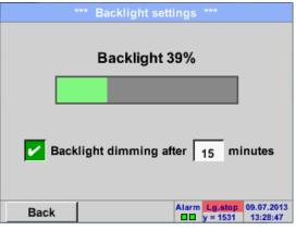
With the help of the *Backlight dimming after* button, after a definable time interval (here after 15 minutes), the *Backlight* can be reduced to the minimum.
