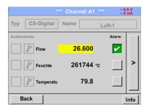
Like in *Main→ Real time values*, individual channels can be selected here, to detect which and how much the value has exceeded or below the alarm range.
