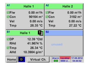
The overview of *Real time values* shows the current measured values of all connected sensors.
