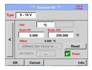
By *Scale 0V* enter the lower and by *Scale10V* the upper scale value
