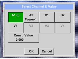
By pressing a button either for HW-, virtual channel or const. Value e.g. *A1* a list of all available measurement channels or measurement values will appear.
