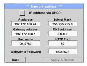
Here you can set up and made a connection, with or without *DHCP*, to a computer.
