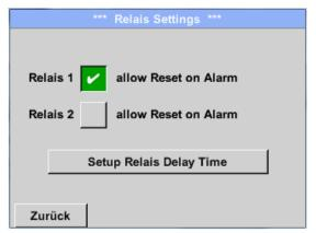
By activated *relais* button it is allowed / possible to turn off the corresponding alarm relays in the popup appearing in alarm case.
