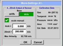
In *More-Settings*, you can define whether the 4 - 20 mA analogue output of the sensor based on the flow rate or velocity.
