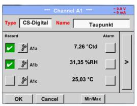
The DS 400 detects, if the connected sensor is a flow or dewpoint sensor of **CS Instruments** and set the CS-Digital subtype automatically correct.
