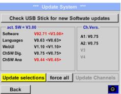
If after pressing the button "Check USB Stick for new Software updates" the following messages appear in the window, is the DS 400 is not properly connected to the USB flash drive or there are no files available.
