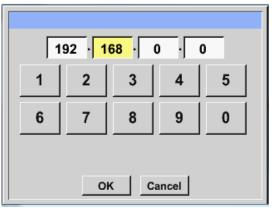
After pushing, for example the *IP address* description field, the command window appears, where in the selected yellow area a partial *IP address* can be entered manually.
