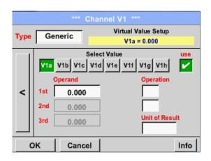
Every virtual value has to activated by selecting the respective *Value-Button* e.g. *V1a* and pushing of the *Use Button*.
