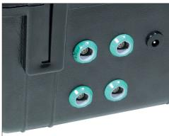
Up to 4 sensors can be connected including power supply for all sensors
