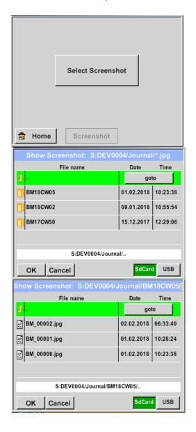
This allows the stored pictures (measurement pictures) on the SD-Card or USB Stick to load and shown in the display again.
