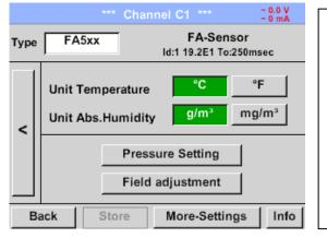
Unit selection for temperature and humidity by pressing the button  $^{\circ}C$ ,  $^{\circ}F$ ,  $g/m^3$  or  $mg/m^3$ .
