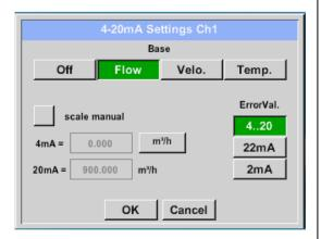
activating the appropriate measured value key in this example, "Flow".
