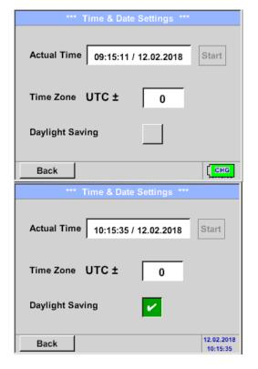
By pushing the *Time Zone* description field and enter the correct *UTC*, you can set the correct time all over the world.
