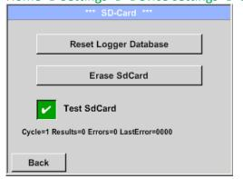
With activation of *Test SdCard* data are written and read to and from the SD-card.
