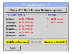
I If the LD 500 is correctly connected to the USB stick and there are new versions of the individual SW Parts, the new versions are marked in red.
