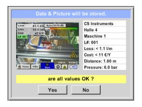
Before final storage of the measurement on the internal SD card, a summary is created and the correctness is queried once more for safety.
