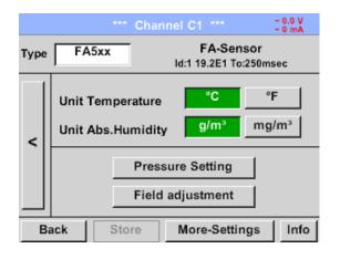
The system pressure is inserted by entering the values in the corresponding text field. The unit can be freely selected, selection menu is opened by pressing the corresponding button units
