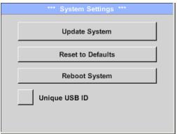
If needed with "Reboot System" the LD 500 could be started(reboot) here.
