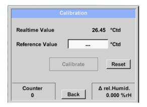
Here, a one-point adjustment can be performed.
