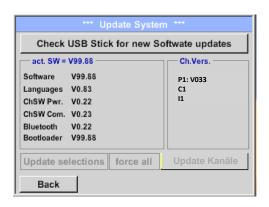
f after pressing the button "Check USB Stick for new Software updates" the following messages appear in the window, is the LD 500 is not properly connected to the USB flash drive or there are no files available.
