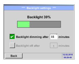
With the help of the *Backlight dimming after* button, after a definable time interval (here after 15 minutes), the *Backlight* can be reduced to the minimum.
