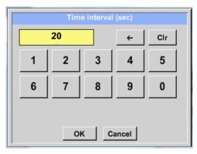
A different, individual *Time interval* can be entered in the highlighted white description field right at the head, where the currently set *Time interval* is always displayed.
