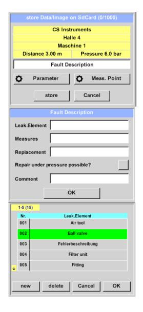
In addition to the details of the measuring point with company, building and location, it is possible to enter a fault decription (up to 32 characters).
