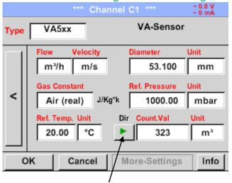
In case of a bidirectional sensor (VA5xxB) can be changed here by pressing the key to switches the other direction and thus the second counter reading is entered
