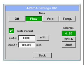
A "manual scaling" needs an activation of the "scale manual" button.
