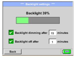
To reduce the energy consumption (device runtime), you can switch off the display backlight by setting "Backlight off after".
