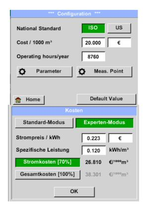
In the configuration settings the unit system can be selected and the required parameters entered, this to calculate the leakage costs per year.
