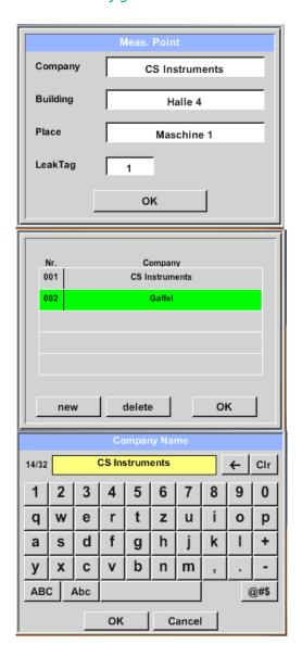
The measuring point is stored for each leakage in its journal data. These can be seen later in the leakage report in the software.
