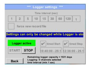
The data logger can be started without activated time settings, use the *Start* and *Stop* buttons for activate and disable.
