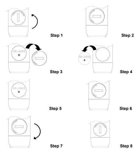
Step1: Turn the battery cover anticlockwise to open it.
