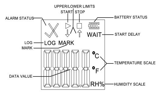
During normal recording process, shortly press "▶" to switch to different display interface. The interfaces shown in sequence are respectively:
