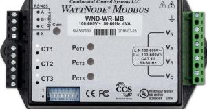
The WattNode<sup>®</sup> Wide-Range Modbus Meter measures bidirectional energy, power, voltage, current, etc. It communicates using Modbus<sup>®</sup> RTU over RS-485. The WattNode Wide-Range provides revenue-grade system accuracy when used with the CCS Accu-CT<sup>®</sup> family of revenue grade (C0.6 or better) current transformers.
