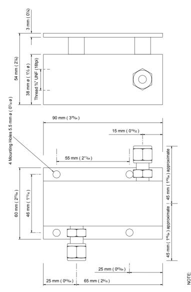
The assembly is shown with 6.35 mm (1/2 inch) OD tube fittings. The dimension across the tube fittings will vary for all other size fittings.
