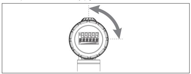
Depending on the conditions of the measuring point, the device can be installed in any other position. The LCD display can be rotated in 90° steps depending on the desired installation position.
