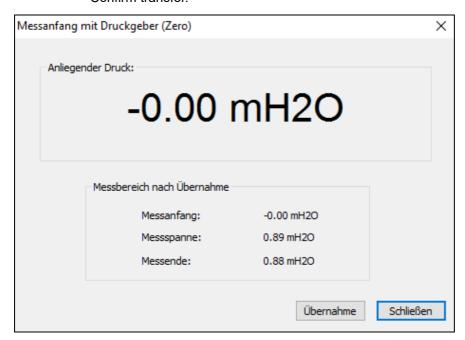
Extras Extras: Online operation\_measuring end with pressure transmitter (span) – with full tank
