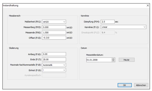
P01 Measuring unit, e.g. mbar P04 Attenuation: 0 P05 Measuring range lower range value: 1461.69, see example calculation P06 Measuring range upper range value: 77.50, see example calculation P11 Characteristic line: linear P14 Temperature measuring unit (only for displaying or as HART® signal): °C P16 Scaling start: scaling on the tank, e.g. in liters: 0 P17 Scaling end: scaling on the tank, e.g. in liters: 200 P18 Maximum decimal place: automatic P19 Scaling unit: L (liters)
