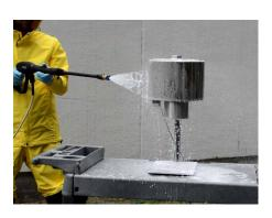
\*As per Keystone Compliance, PA Testing; ENVIRONMENTAL TEST REPORT 1712-067NA-1 REV. N/C, TEST STANDARDS: IEC 60529.
