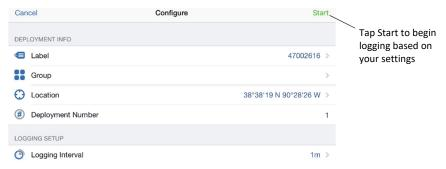
**Important**: If the connection is lost between the logger and your phone or tablet before tapping Start, you will need to reconnect and reconfigure the logger. Configure settings are not loaded onto the logger until you tap Start.
