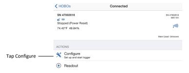
7. Make your selections and then tap Start in the upper right corner of the Configure screen. The logger will begin logging based on the settings you selected (see Chapter 2 for details on settings).
