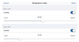
3. Enable Low Limit if you want burst logging to occur when the sensor reading falls below a specific reading. Drag the slider to the reading that will trigger burst logging or tap the value field and type a specific reading. In this example, the logger will switch to burst logging when the temperature falls below 32°F.
