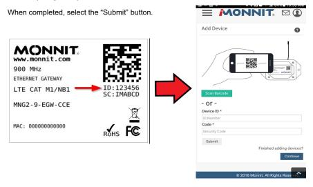
**IMPORTANT:** Add the gateway and all sensors to the iMonnit portal so that on boot, the gateway can download and whitelist the sensors from the configured sensor network.
