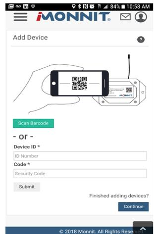
**IMPORTANT:** Add the gateway and all sensors to the iMonnit portal so that on boot, the gateway can download and whitelist the sensors from the account.
